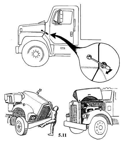
them around. Illustration 5.11 shows a typical hood lock and a couple of hood configurations. Many truck hoods are made of lightweight plastic or fiberglass and are easily opened. As illustrated, handles, and even hood ornaments, are used to open hoods for access to the engine. Look closely at some trucks, as if out of curiosity, before attempting clandestine access.
