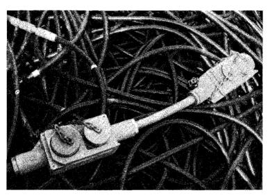
Seismic cable. Note cableheads.
