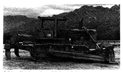
Bulldozer. Note the smoke stack (exhaust pipe).
