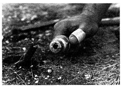
Note the "seat" created in the end of the driver (the  $\frac{1}{4}$  inch nipple screwed into one of the reducers).
