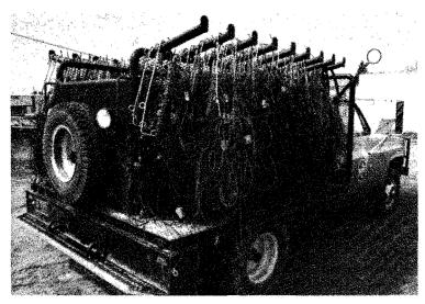
Truck with seismic cable.
