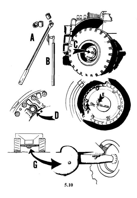
Various types of oil filler caps found on wheel hubs can be seen in (C) through (F).
