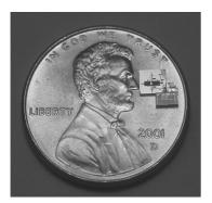
information back to a central command with enough computing power to crunch the data. The target size for Smart Dust "motes" is 1mm cube, increasingly approximated by existing developments (illustrated left on a 1¢ coin – cf. Warneke 2004), and it is a safe bet that
